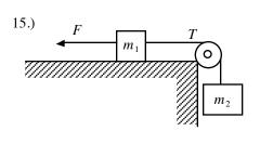
In the figure to the left  $m_1 = 35$  kg and  $m_2 = 25$  kg. The coefficient of kinetic friction is 0.15 between  $m_1$  and the surface. A force F = 600 N is applied to  $m_1$  causing it to accelerate to the left.
